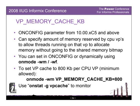
ONCONFIG parameter VP\_MEMORY\_CACHE\_KB -- specifies the amount of private memory blocks of your CPU VP, in KB, that the database server can access. The cpu vp private memory is allocated from IDS shared memory. Acceptable values are: 0 (disable), 800 through 40% of the value of SHMTOTAL.
