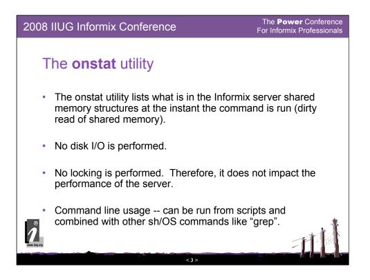
The **onstat** utility reads the server shared-memory structures and reports the contents of shared memory at the *instant* that it is run. This means the contents of shared memory might be changing as **onstat** results are printed (as no memory locking is done by **onstat**).
