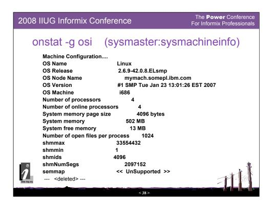
onstat -g osi is a useful onstat that displays common machine configuration info and kernel parameters. The same information can also be obtained from sysmaster:sysmachineinfo pseudo table.
