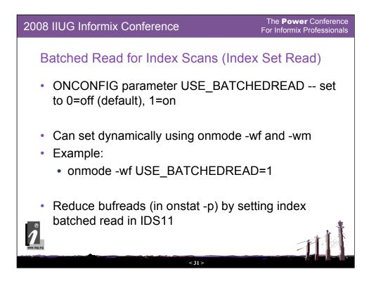
USE\_BATCHEDREAD for index scans was introduced in IDS 11 (11.10). Can monitor with onstat -g idxscan and onstat -p (look at bufreads).
